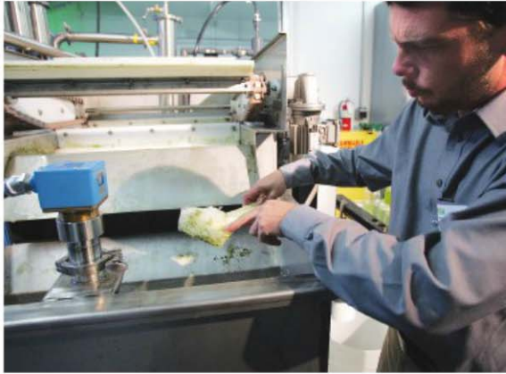
6 Gavin Gray, OriginOil's senior director of engineering, scoops up a spoonful of algae crude. The algae appliance uses tiny air bubbles to lift broken-up algae out of water, giving the algae a frothy consistency.
