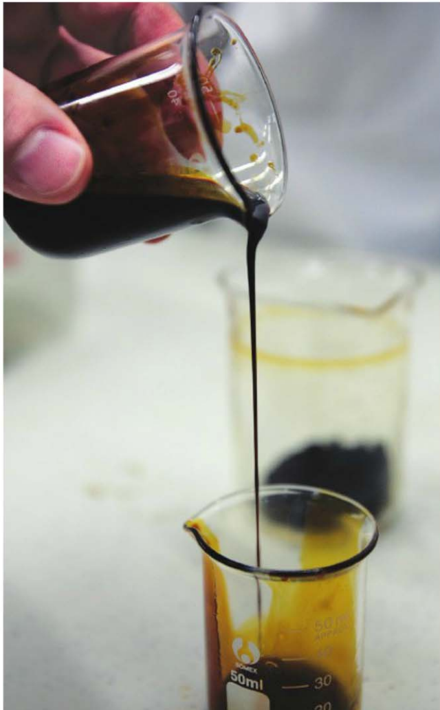
10 After other processes, OriginOil's algae crude is turned into bio crude, shown here. Bio crude is similar to standard crude oil and can be processed into gasoline and other petroleum products. The company is working with the Idaho National Laboratory to make that process feasible on a large scale.
